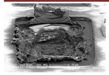
Some of the damage Caltech engineers intentionally inflicted on their self-healing power amplifier using a high-power laser. The chip was able to recover from complete transistor destruction. This image was captured with a scanning electron microscope.
