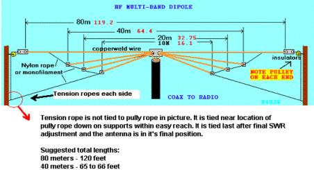
80 meters - 120 feet 40 meters - 65 to 66 feet 20 meters - 34 feet 10 meters - 17 feet These lengths are not exact. Some tuning may be required. Use the standard formula 468 / freqmhz for total feet for each band (freq) of interest. Adjust each length longer or shorter as needed.
