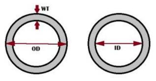
3. One can completely specify a piece of pipe/tube by supplying any two of these numbers.
