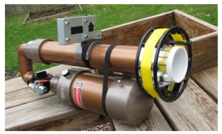
As an amateur radio enthusiast, [Andrew] sometimes has to set up impromptu antennas up to 160 meters in length. The easiest way to get these antennas off the ground is to drape them over trees, a feat normally accomplished by lofting fishing line into the air with a slingshot or bow and arrow. [Andrew] thought slings were *so* last century, so he came up with a <u>spud gun</u> inspired antenna launcher.
