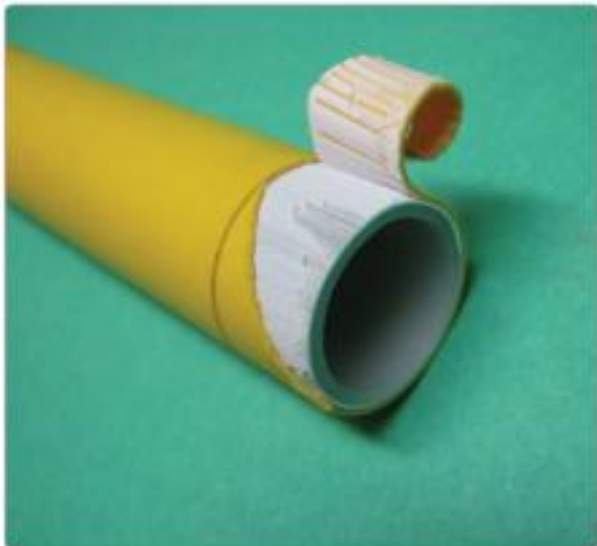
Photo 2: Stripping the end of the plastic pipe.
