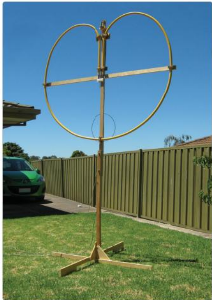
Photo 1: The completed magnetic loop.
